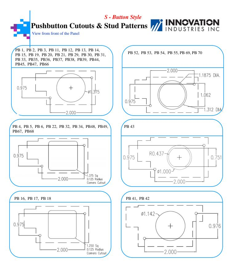
All Studs are 6-32 x 1.0625" long. Stud patterns can be rotated 90 degrees for vertical mounting.
